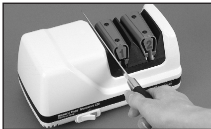
Figure 3. Stage 1. Inserting blade in slot between guide and elastomeric spring. Alternate individual pulls in left and right slots.
